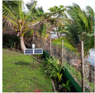
Continuous monitoring network based on Cairsens sensors
