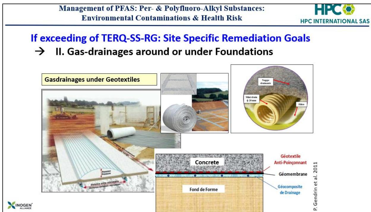
Fig. 17a-d: Constructive Measurements by Gas Drainages to avoid FTOH & COV vapor intrusions into building's ambient air by drainages pipes and drainages carpets, Gendrin et al. 2011.
