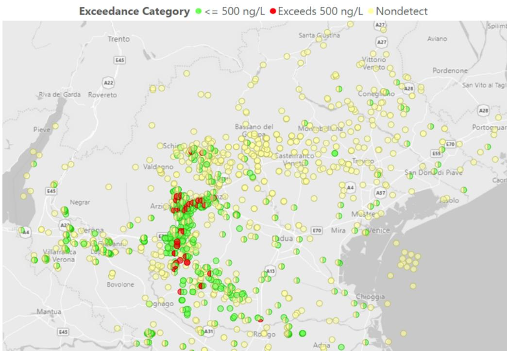
Figure 3: distribution of PFBA concentrations in the surface waters and groundwaters of the study area
