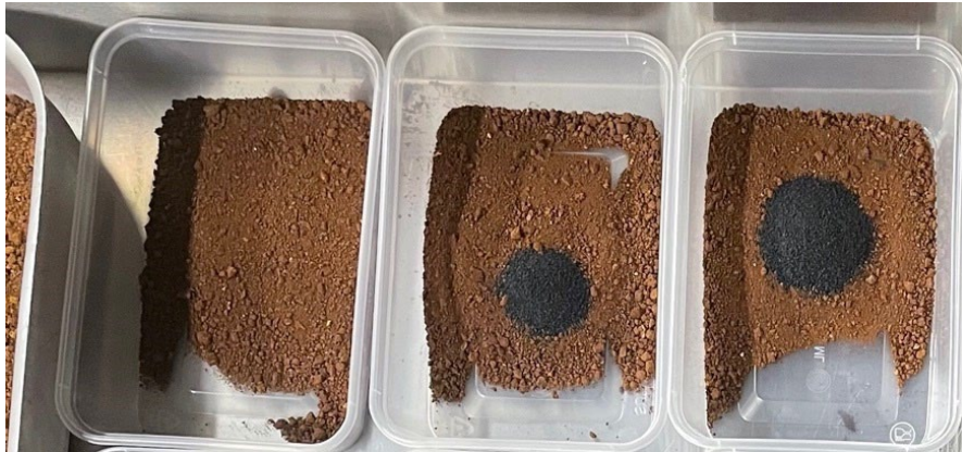
1. Screen soil, dose reagents (0% to 5%)
