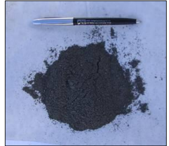
Granular EHC powder – composed of microZVI and solid plant fibers
