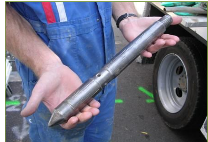
Injection probe with check valve
