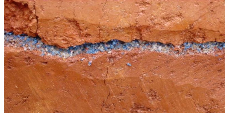
Sand seam emplaced via hydraulic fracturing (courtesy of FRx)
