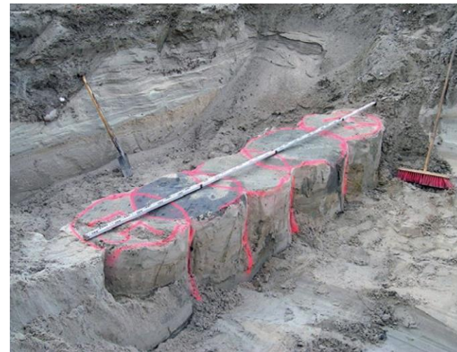
Cut-off wall with DSM, dike in Germany
