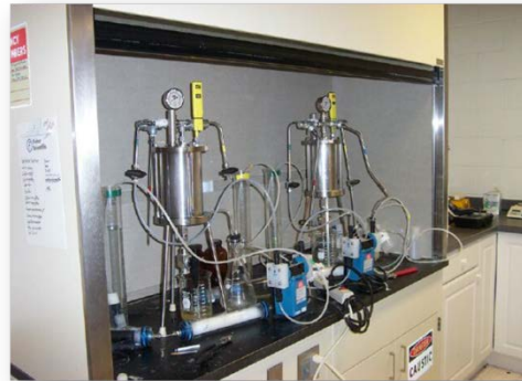
Fig 2-1: Titration of Slurry – Core zone
