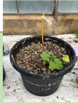
Reconstructed soil 2 30% treated sediment + 70% agricultural soil Tr_Sed+Soil
