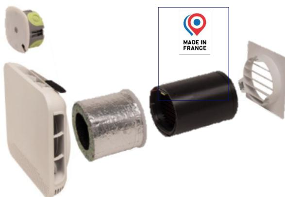
In order to match French regulation on air inlets, the filter is an electrostatic precipitator (ESP). The air gets through a set of ionizers and then a system of polarized parallel plates where particles are collected. The air openings are never below 4 mm. The pressure drop of the filter in itself is around 1 Pa.
