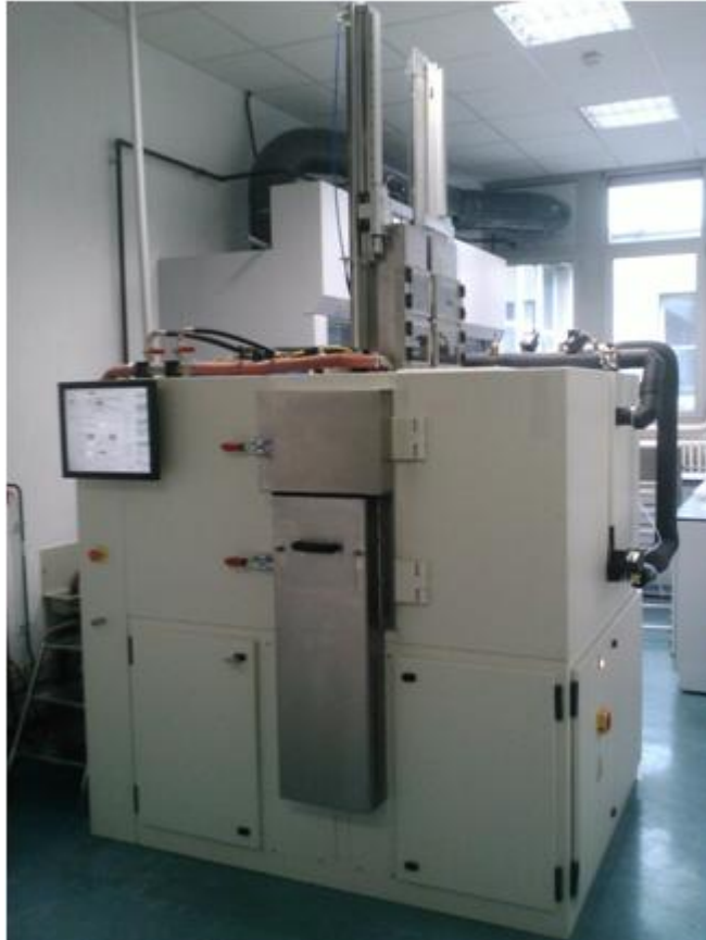
Environmental chamber, 1m 3 Pressure, T° (10 - 40°C), RH (20 – 80 %), air velocity (0,1 - 2 m/s), calibrated gas control
