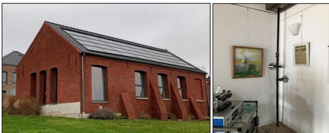
**Figure 1: Installation of the FLEC for surface emission measurements at the town hall of Moncheaux**
